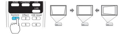
Your projector automatically adjusts images that look like \_\_\_\_ or \_\_\_\_, but if necessary you can press the **Keystone** button to correct it.
