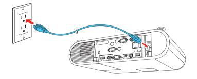
3 Press the  $\bigcirc$  power button on the remote control. The projector beeps, the status light flashes blue, and then stays on.
