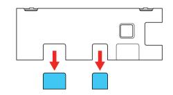
2 Attach the interface cover on the projector as shown.
