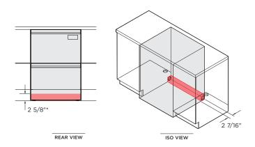
Service outlet at rear extends both sides, hoses and cords can be routed to either or both sides. Units shown in inch. \*depending on adjustment of leveling feet
