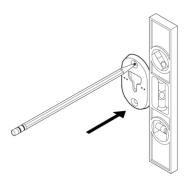
If you're using wall anchors, use a 5/16" drill bit to drill 2 pilot holes, starting with the hole on the top. Then insert the wall anchors. (Don't use wall anchors if you're drilling into wood or plastic.) If you're not using wall anchors, locate a wall stud and drill the pilot holes with a 9/64" bit.
