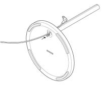
Use the alignment pins to position the speaker platform on the pole, then attach the speaker platform to the stand pole using the other long screw (included).
