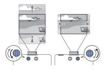
If the projector is on a table, you can level the image by turning any of the projector's adjustable feet.
