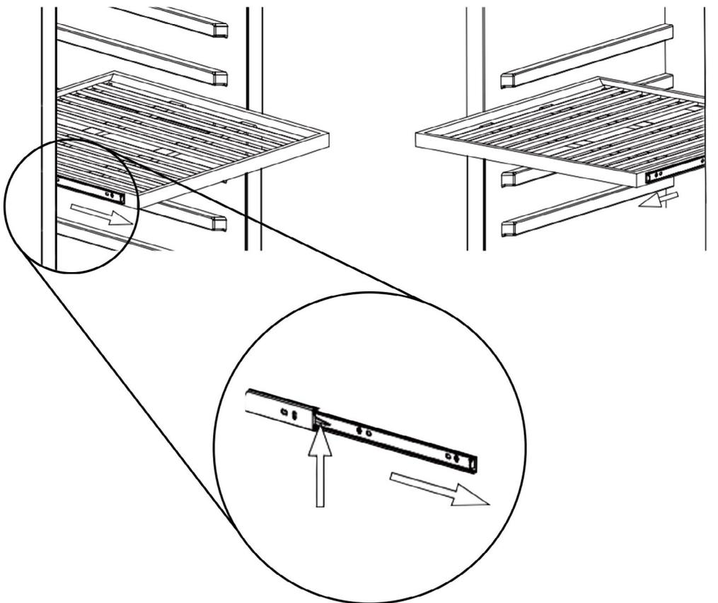
**Note:** These installation instructions are for wooden shelves that come with the dual zone wine cooler. ZLINE beverage coolers are equipped with glass shelves. To adjust or remove, open the door completely and simply slide the shelves in and out of the pre-installed metal brackets on the beverage cooler.
