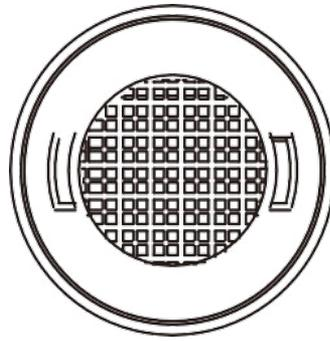
To replace the filter, first remove racks/shelves from the top of the unit to access the filter. Then, using a pair of needle-nose pliers, stick the ends into the slots on each side of the filter, turn either clockwise or counter-clockwise until the slots are at the top and bottom, and then pull out the filter from the rear panel. Put the new filter in and reverse the order.
