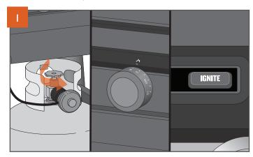
Make sure the propane tank valve has been turned to the fully open position. Turn the knob for the desired zone to the ignite position (\*). Press the IGNITE button and hold until you see the flame sensor light illuminate. Once the flame sensor has illuminated, ignition is successful.
