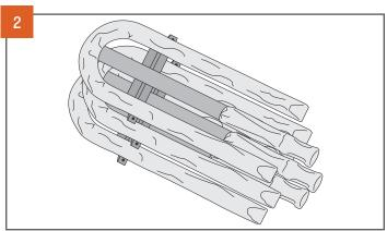
When storing the Flat Top Grill or before an extended period of nonuse, remove the burners and wrap them with aluminum foil to reduce the risk of insects entering the burner holes.
