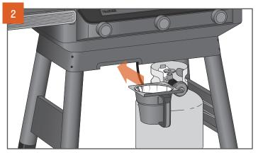
Empty and discard the keg liner. Line the EZ-Clean™ Grease Keg with a new liner and slide it back into the bracket on the bottom of the Flat Top Grill (you will feel it "drop" into place when installed fully).
