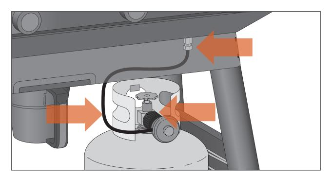
Perform a leak test after a new tank is added, after service, or following a period of non-use to ensure that there are no gas leaks. In addition, whenever the gas tank is connected to the regulator or whenever any part of the gas system is disconnected or replaced, perform a leak test.
