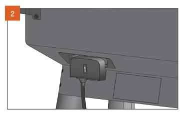
Set the main power switch on the back of the grill to ON (I). The power switch will illuminate when turned on.
