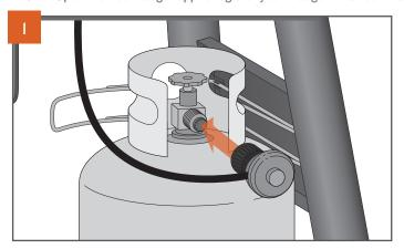
Be sure all control knobs are in the OFF (O) position. Screw the end of the regulator onto the propane tank valve. Hand-tighten.
