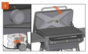
Turn all knobs to the OFF (o) position, close the lid, and turn the propane tank valve closed. Always shut off the propane tank valve completely after every cook.
