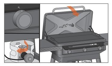
Turn all knobs to the OFF (o) position, wait until the cooktop is cool, close the lid, and turn the propane tank valve closed. Once the flame sensor light is off, the Flat Top Grill is no longer on and will start cooling down.
