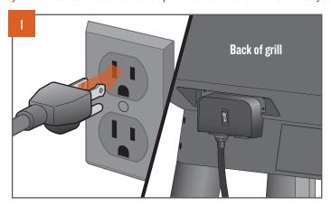
Plug your grill into a grounded electrical outlet and set the main power switch on the back of the grill to ON (I). The power switch will illuminate when turned on. Make sure you have your propane tank nearby for the next step.
