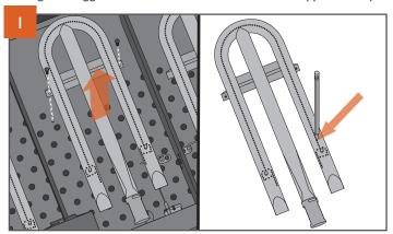
Remove burners from the Flat Top Grill by unscrewing the two fasteners on the burner brackets. With burner removed, insert a pen tip or paperclip into the clogged burner inlet hole to clear out any debris that may have accumulated.
