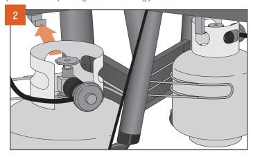
With the regulator connected to the tank and the fuel sensor calibrated, lift the tank onto the hook beneath the Flat Top Grill. Any of the holes or handles in the tank collar can be used as hanging points. Make sure that the tank is fully seated on the hook and resting against the tank back brace.
