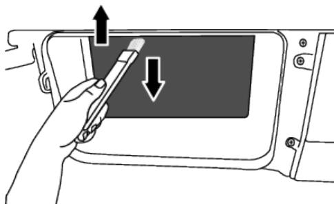
**Sharp Edges – To reduce the risk of injury, use care when cleaning the condenser or evaporator coil fins.** You can clean by hand, provided you wear protective gloves. Do not try to clean with bare hands. The condenser fins may damage your hands. Cleaning from left to right may damage the condenser fins. This may lead to drying issues.
