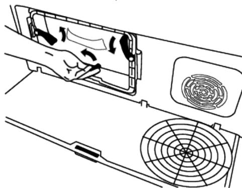
Pull the brush to the left to remove it. You can use the cleaning brush to clean filter, condensing metal surface and accumulated fibre on the door.
