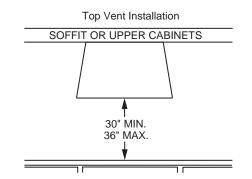
In this installation, the ductwork running from the top of the hood will be concealed in the soffit or upper cabinetry.
