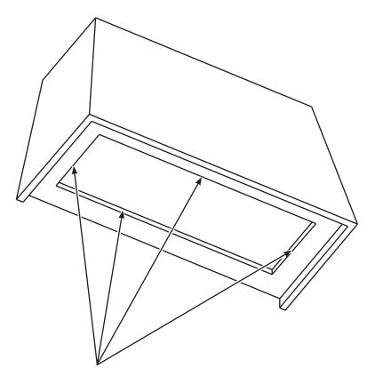
Use provided screws to attach the Insert to the Hood as directed in the Insert Installation Instructions.
