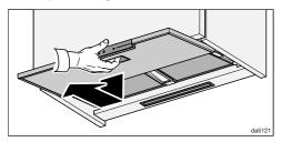
■ Pull out the canopy. To ensure optimum extraction and a low noise level, pull the canopy all the way out.
