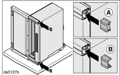
■ Insert the depth stops into the recesses of the deflector plate from behind. The alignment is determined by how far forward you wish to move the stop.
