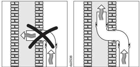
If the exhaust air is to be ducted into a flue, the ducting must be directed in the flow direction of the flue.
