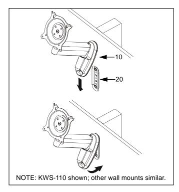
Figure 2: Install Wall Mount
