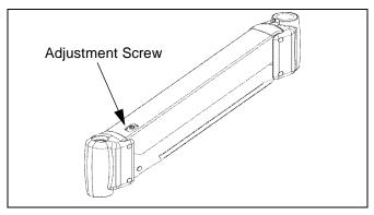
Figure 25: Height Adjustable Arm Adjustment
