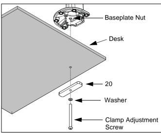
Figure 8: Desk Mount - Hole Installation
