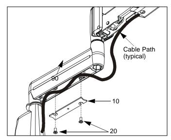
Figure 23: Static Arm - Cable Path
