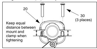
Figure 10: Securing Pole Mount and Clamp
