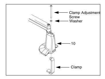
Figure 7: Remove Clamp Adjustment Screw
