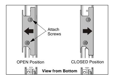
Figure 21: Height Adjustable Arm - Cable Management Bracket
