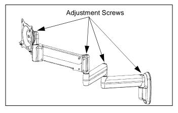
Figure 24: Pivot / Swing Arm Adjustment
