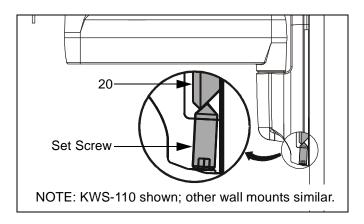
Figure 3: Tighten Set Screw
