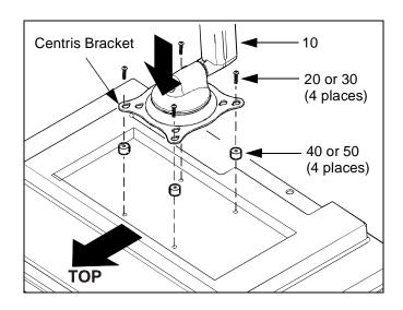
Figure 12: Single Display - Recessed Mount
