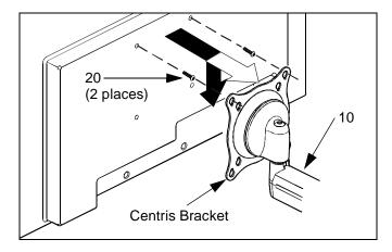
Figure 11: Single Display - Flush Mount
