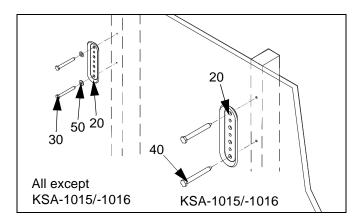
Figure 1: Install Wall Bracket
