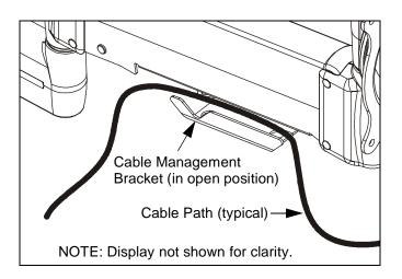
Figure 22: Height Adjustable Arm - Cable Path
