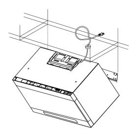
Bertazzoni recommends to operate the appliance after it has been installed in a cabinet. The kitchen cabinets shall be made of materials capable of withstanding temperatures at least 117°F (65°C) above room temperature in order to avoid possible damage to the cabinets during oven usage. For further installation instructions refer to the installation manual.
