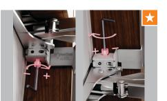
Open the door and use the supplied hex key to expand the spacers. Ensure no gaps are present.
