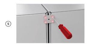
Secure the bracket at the rear top using four screws.
