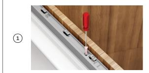
Fit the top cover using two screws. Ensure flat side faces out from the panel.
