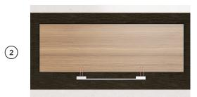
Ensure all bracket and handle holes have been pre-drilled. Refer to 'custom panel preparation' for details.
