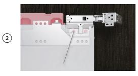
Carefully remove hinges from door and set aside. Remove top cover and set aside.
