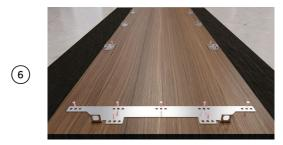
Using the screws supplied in the install kit, secure the door panel bracket using seven screws.
