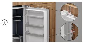
Remove the flow divider and panel bracket before removing all door panel side screws and the M8 washer and nut. Lift panel up and out to remove.
