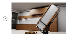
Tilt product onto handtruck and remove palette. Move product to the installation location. Remove and discard corner posts.
