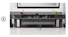
Open the cover and align the grille to the product. Slot into place starting with the base of the grille. Hand tighten the top left screw first, followed by the top right screw. Fit the remaining five screws on the grille to secure.
