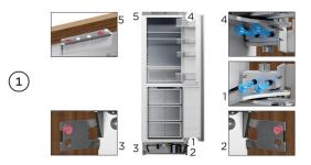
Open the door and secure following the sequence shown. The longer screws should be used where shown in blue, and the smaller screws where shown in red. Ensure a gap between drill and product is maintained to avoid cosmetic damage.
