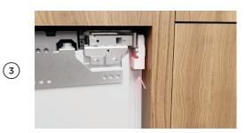
Clip covers onto spacers. Ensure cover A is fitted to spacer A and cover B to spacer B.
