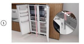
Locate trim between products. Lower trim before pushing in to ensure bottom connector bracket clears the grille. Slide trim up until it slots into the top bracket.
