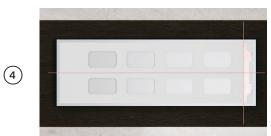
Determine the panel orientation based on the hinge and handle positions. Red labels indicate left hinge installations, blue labels indicate right hinge installations.
