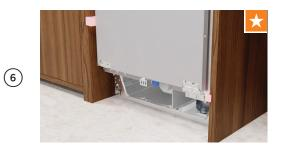
Push product into alcove. Push in until the gauges touch the alcove end. Ensure hose doesn't bend or kink and that the power cord is not trapped.
