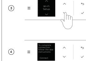
Press ✓ or ∧ to scroll through the list and select WI-FI SETUP. Press ✓ to confirm.
