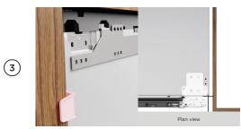
Ensure all depth gauges are flush to the front of the alcove.
