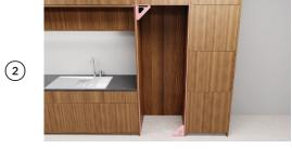
Check alcove is square and is secured to the wall. Ensure front of alcove is square to the top of the alcove and the floor is flat.
