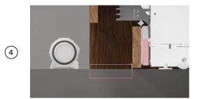
Push the toe kick back to the desired depth before removing. If toe kick depth is less than 3 9/16" (90mm), attach the additional foam block.
