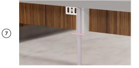
Cut the seal to length and clip onto the front of the flow divider. Ensure tabs on the seal and flow divider align.
