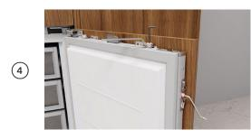
Fit side screws to panel using the short crosshead tool provided in the install kit. For 90° door opening installs, the supplied crosshead key should be used on the hinge-side.
