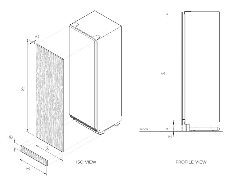
NOTE: Left hand hinge is a mirrored version of the image shown. Left hand hinge can be achieved using supplied parts.
