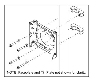
Figure 2: Vertical Pole Installation (Typical)
