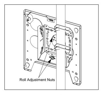
Figure 11: Roll Adjustment
