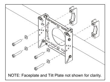
Figure 3: Horizontal Pole Installation (Typical)
