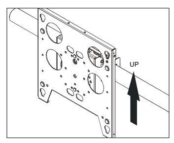
**Figure 5: Horizontal Mount Orientation**
