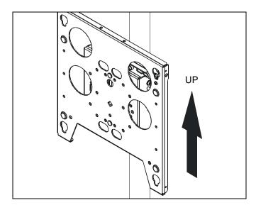
Figure 4: Vertical Mount Orientation
