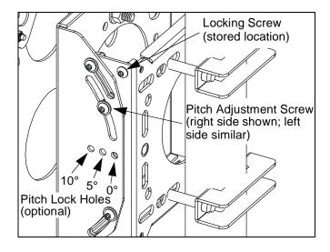
Figure 9: Pitch Adjustment
