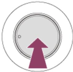
The menu is displayed, and you can perform input selection and various settings by moving the joystick up, down, left, and right.
