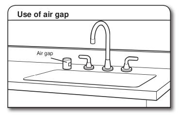
If required, the air gap should be installed in accordance with the air gap installation instructions. When you are connecting the air gap, a rubber hose (not provided) will be needed to connect to the waste tee or disposer inlet.
