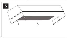
Reinstall the main liner plate to the base of the custom hood and secure it with (5) 3/4" screws.
