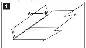
Install 1 small pad (A), included in the hardware package, to each side of the main liner plate. (See figures 1 and 2)
