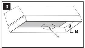
Using a pen, mark the outline of the future opening for the power pack. Remove the main liner plate (**B**) from the custom hood.
