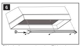
Slide the front panel section (**D**) into the nose of the custom hood base. Take care not to scratch the main liner plate when installing the front panel section of the liner. Assemble it to the cabinet using (3) 1/2" screws.
