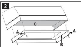
Temporarily install the main liner plate (B) to the external base of the custom hood (C). When inserting the main liner plate, push slightly on the pads (A) to prevent damage. Main liner plate should be positioned as far back as possible.
