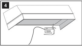
Cut out an opening in the bottom of the custom hood.
