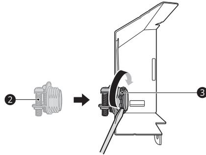
**6** Insert the electrical cable through the hole in the strain relief. Tighten 2 screws to secure the cable.
