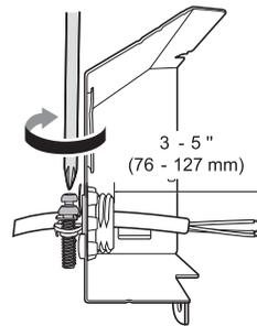
**7** Pull the existing wires through the openings in the junction box. Tighten 2 screws **4** to reassemble the junction box in the appliance.
