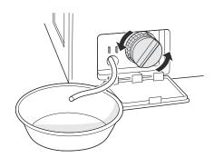
**5** Clean the pump filter and opening.
