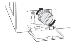
Close the drain pump filter cover.
