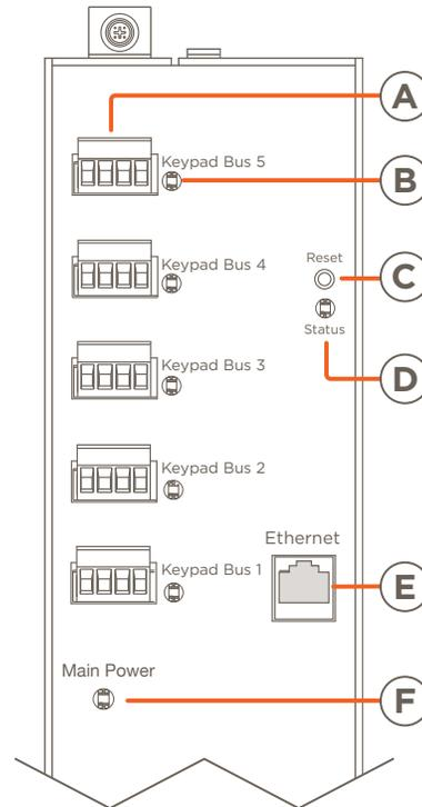
**A Keypad Bus (1-5)** - Up to 10 low voltage keypads wired in a daisy-chain fashion are supported per keypad bus with a maximum of 40 keypads per power module.
