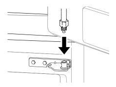
**2** Fit the hinge **1** over the hinge lever latch **2** and slot it into place. Rotate the lever 3 counterclockwise to secure the hinge.
