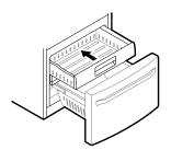
**5** Replace the ice bin in the drawer. Insert the Durabase basket in the rail assembly.
