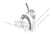
5 Hold the water supply connection and gently push in the collet 4 to connect the water supply line as shown. Insert the tube at least 5/8 inch (15 mm) into the connector. Insert the clip on the joint to fasten the tube in place.
