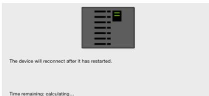
7. After reboot, the screen defaults back to the **Firmware** screen. **DO NOT** remove cable at this time. Firmware is now installing into the CLI-8000. Firmware will take about 4 - 5 minutes to install. Once installed, the CLI-8000 will automatically reboot. Wait for it to finish the complete boot process. Once the main menu is displayed again, the system can be disconnected.
