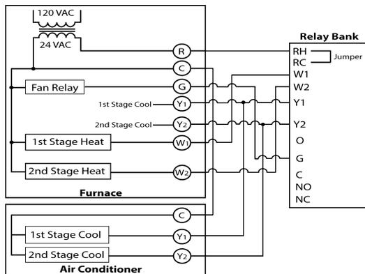
Two stage HVAC system that supports both heating and the air conditioning.
