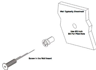
7. Feed the remaining wires back behind the wall and press the sensor into the wall anchor until it is flush.
