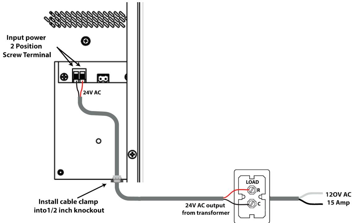
4. Connect the other side of the transformer to a 15 Amp (minimum) circuit. It is recommended that the CLI-8000 be connected to its own circuit.
