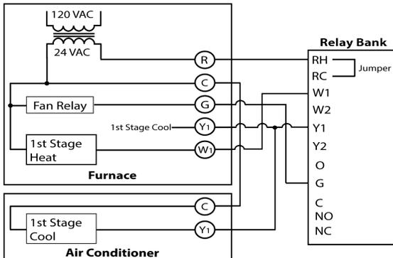
Single stage HVAC system that supports both heating and air conditioning.
