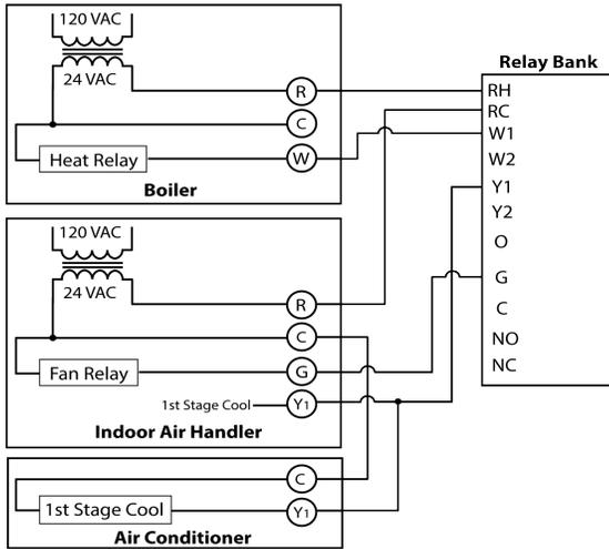
This system uses a boiler for hot water and possibly radiant or baseboard heat. The air handler is used in conjunction with the air conditioner for cooling.
