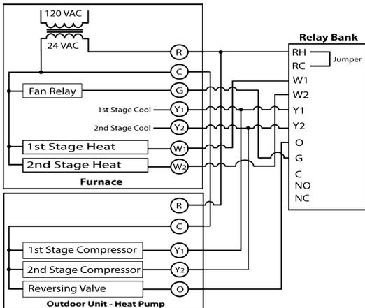
This system uses an indoor air handler with condenser for supplying heat and an evaporator for supplying cool. The system has a reversing valve to select whether heated or cooled air is produced. The system has two stage heating as well as two stage cooling.
