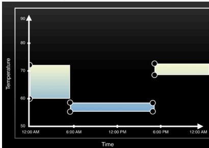
The schedule above is a fall schedule where the temperature from 12:00AM to 6:00AM is set to not go below 60°F and not go above 72°F. From 6:00 AM to 5:00 PM the temperature is kept between 55°F and 58°F. At 5:00 PM the temperature is set to stay between 68°F and 72°F
