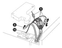
Rotate the hinge lever **10** counterclockwise. Lift the top hinge **②** free of the hinge lever latch **B**.
