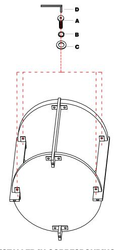
NOTE: DO NOT TIGHTEN ALL THE BOLTS UNTIL THEY ARE INSTALLED IN CORRESPONDING HOLES!
