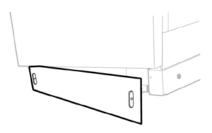
The kick plate can also be installed with magnets.
