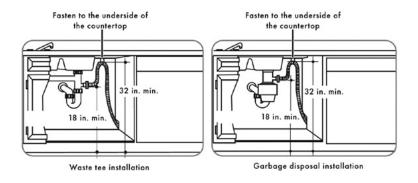
4. If connecting the drain line to a garbage disposal, make sure that the drain plug has been removed. Your dishwasher will not drain if the plug is left in place.
