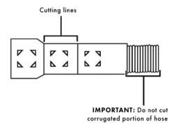
2. If a longer drain hose is required, you can add up to 42" of length, for a total of 10 ft. to the factory installed hose. Use 5/8" or 7/8" inside diameter hose and a coupler to connect the two hose ends. Secure the connection with screw-type hose clamps.
