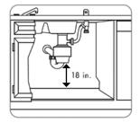
Method 2 - High drain with a waste tee or garbage disposal connection
