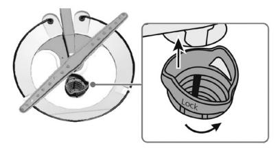
3. Lift the fine filter from the bottom of the tub.
