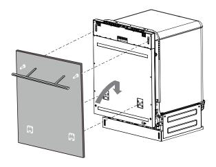
4. Fix the decoration door onto the outer door by screws.
