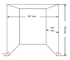
If installing into a corner, allow 2 in. min. clearance between dishwasher and adjacent cabinet, wall, or other appliances. Allow 25.63 in. min. clearance from the front of the dishwasher for opening the door.
