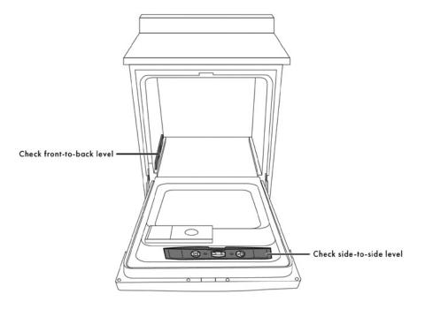
2. Level the dishwasher by adjusting the three leveling legs individually.
