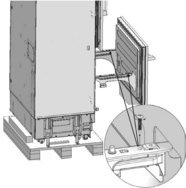
While supporting the door, pull it forward while freeing it from the rear rail lock tabs to remove it.
