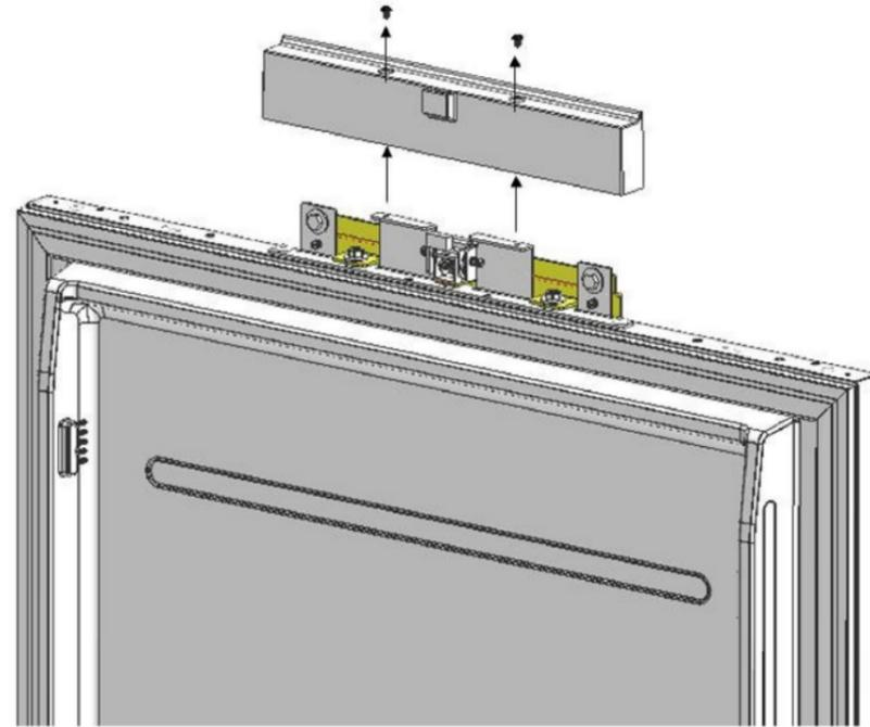
Note: There is a magnet in the cover of the top refrigerator door hanger bracket. This is a functional part for the operation of the product.
