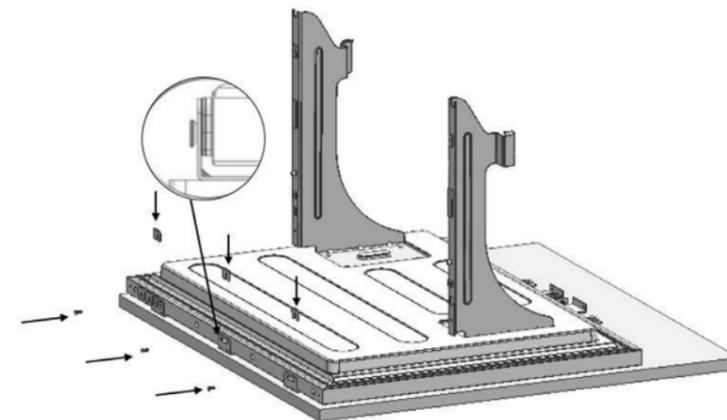
A total of (3) 1 mm washers must be placed on the freezer door on the condition that all door panel dimensions are suitable. Washers to be used are determined based on the kitchen design.
