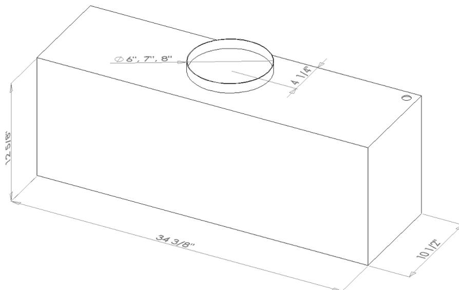
Note: Electrical access located on the top, right side as shown in the above dimensioned diagrams.
