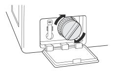
Close the drain pump filter cover.
