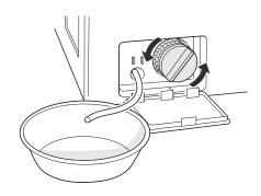
Clean the pump filter and opening.
