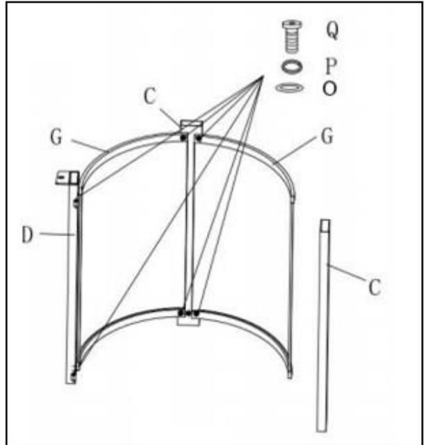
2. Secure the side(G), back post(C), ignition side(F),front left side(E) with 6pcs 1/4in x 20mm bolts(Q),6pcs spring washers(P) and 6pcs flat washers(O) .
