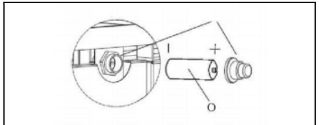
9. Open the door, place the 20-pound cylinder into the main body and tighten it as shown on the right, so the gas cylinder cannot move and fall down, close the door, put the Burner Cover on the fire pit table top, then cover the fire pit with PVC cover (L) when not in use to protect it from the elements or when fire pit is cool COMPLETELY after the use.
