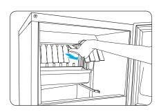
3. Slightly lift the ice slide to remove it.
