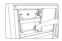
\* Press the switch to set it to (WASH) when cleaning the product; this will repeat the process of supplying water for about 2 minutes and operating the circulation pump 3 times, enabling easier cleaning.
