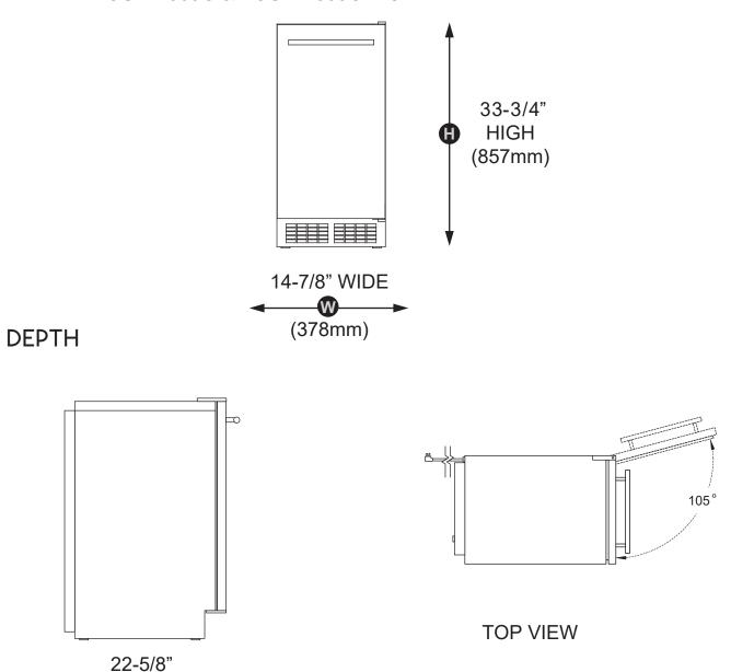
THE OVERALL DEPTH SHOWN (22-5/8") INCLUDES THE DOOR WITHOUT HANDLE. THE HANDLE ADDS 2-1/4" TO THE DEPTH.
