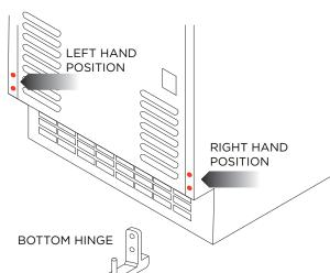
2. Remove the two (2) screws that hold the Bottom Hinge in place. Remove the two (2) corrosponding screws on the left hand side. Install the Bottom Hinge in the left hand position and install the remaining two (2) screws into the holes on the right hand side.
