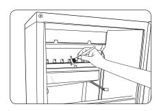
6. Lift the drain connection inside the vessel sheet (water tank), clean it, and drain the water.
