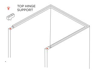
4. Remove the Top Hinge Support which is held in place by one (1) screw from the right hand side and transfer it to the left hand side re-attaching it with the screw.
