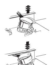
**IMPORTANT:** If the vent is obstructed by an object while it is being raised or lowered, it will stop. Remove the obstruction and press the **ON/OFF** pad again.
