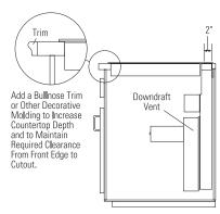
When the distances between the vent and the inside cabinet side walls are more than 5-1/2" and/ or the inside cabinet back wall is more than 4-1/2", false walls should be constructed inside the cabinet for securing the vent with the stabilizing brackets (refer to Cutouts and Clearances under Installation Preparation.)
