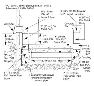
Install ductwork so the piece of duct nearest the downdraft unit slots INTO the next piece of the duct. Secure the joints with self-tapping screws and apply duct tape around the joints to ensure an airtight seal.
