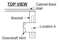
Onfirm the vent system is plumb and square with the cabinetry.
