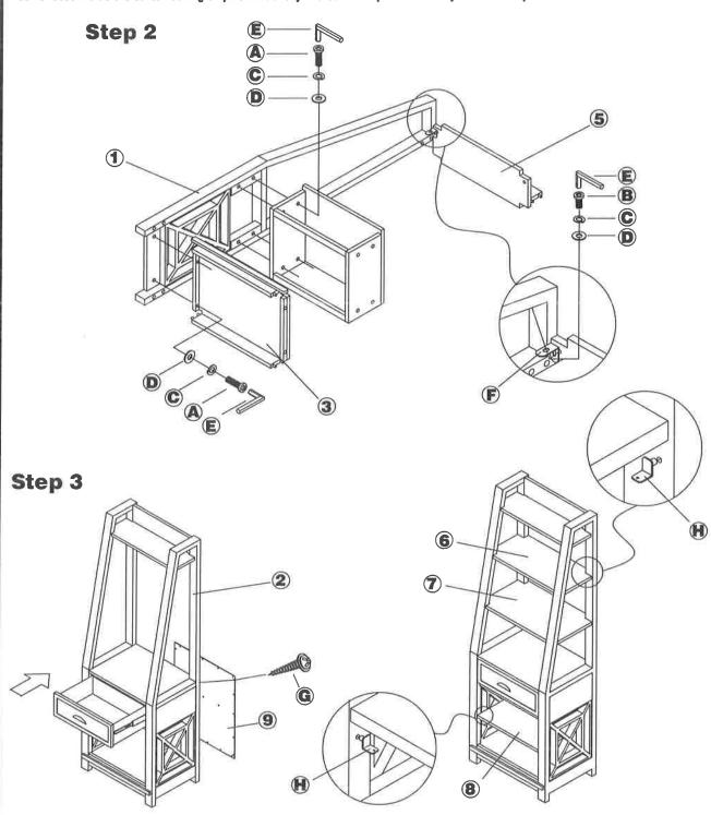
NOTE: DO NOT TIGHTEN ALL THE BOLTS UNTIL THEY ARE INSTALLED IN CORRESPONDING HOLES!
