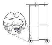
1 Open the door and use the wrench to loosen the keeper nut by turning it to the left.
