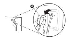
**3** Pull out the water supply lines **7**. Disconnect all the wire harnesses **3**. Unscrew the ground wire **9**.
