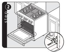
Fold latches backward until locked in place.
