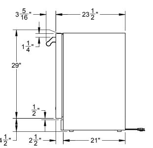
\*- Leg levelers can add  $\frac{3}{4}$ " to these dimensions when fully extended
