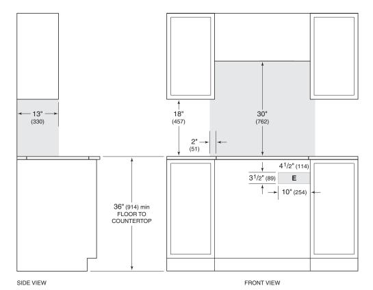
NOTE: Shaded area above countertop indicates minimum clearance to combustible surfaces, combustible materials cannot be located within this area. Electrical supply location only applies to installations with built-in oven.
