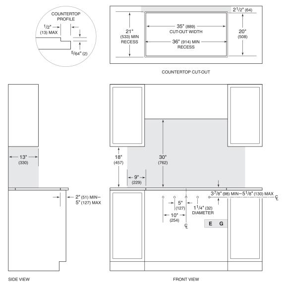
NOTE: Shaded area above countertop indicates minimum clearance to combustible surfaces, combustible materials cannot be located within this area.
