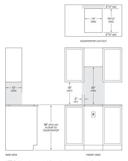
NOTE: Shaded area above countertop indicates minimum clearance to combustible surfaces, combustible materials cannot be located within this area.
