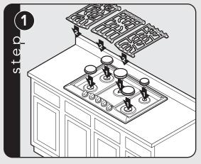
Replace the burner caps and grates. **Note:** The narrow edge of grate goes toward center of unit.
