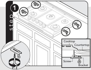
Screw hold down brackets using the  $#10 \times 1/2"$  sheet metal screw to the burner box. (2 brackets per side)
