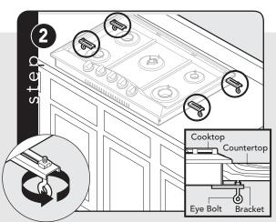
Screw the eye bolt into the self-retaining nut and tighten firmly against bottom of countertop.
