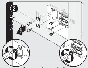
Remove supply cord strain relief bracket and three supply cord mounting screws
