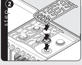
Burner heads and burner caps are packed in the cardboard top pack with the grates. Align burner head on burner base. Place burner cap on burner head.
