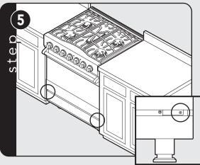
If the door needs to be adjusted, loosen hinge trim screws located in Step 2. Adjust the screws located between the door and kickplate using a 5/32" hex head Allen wrench.
