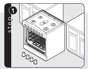
Legs are packed in the cardboard top pack. **Note:** Legs should be installed near to where appliance is to be used, as they are not secure for long transit.
