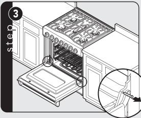
Remove pins from holes in hinges.
