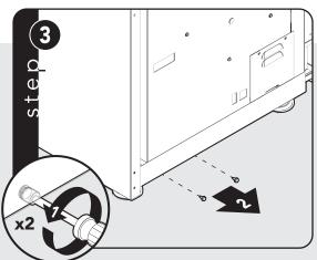
Remove two screws from back of range.
