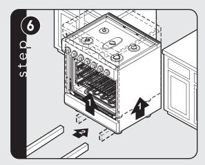
Lift unit and prop on wood blocks.
