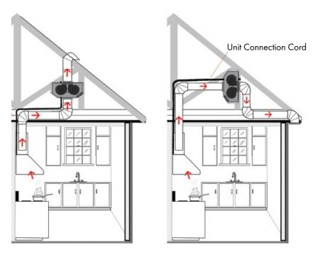
The Remote Blower is designed for our Remote Range Hoods. This unit is installed remotely in the interior of your home. This provides venting, but with reduced noise.
