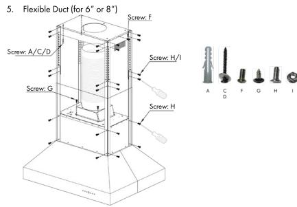
NOTE: Island range hoods with single motors will come with a square to 6" round transition piece and will include a back draft damper. The ducting with these range hoods is 6". Dual motor wall hoods will come with a square to 8" round transition piece without a back draft damper. The ducting with these range hoods is 8" in diameter.
