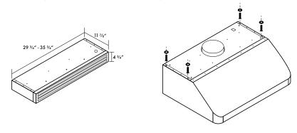
3. Secure the recirculating kit with the provided screws. Once secure, begin tightening each screw until the recirculating kit is flush with the range hood.
