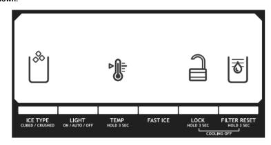
For your convenience, your refrigerator and freezer controls are preset at the factory. When you first install your refrigerator, make sure that the controls are still set to the "mid-settings." The factory-recommended set points are 37°F (3°C) for the refrigerator and 0°F (-18°C) for the freezer.
