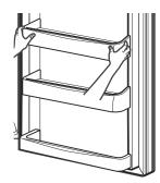
To assemble the bin, slide it in above the desired support and push down until it snaps into place.
