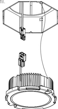
**13** Place module into junction box, aligning screws with washers to screw holes in junction box bracket. Screw to junction box.
