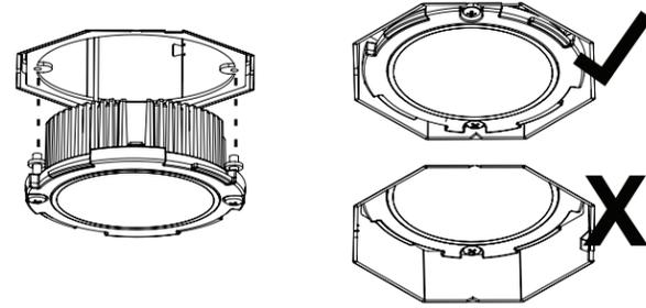
**14** Align trim onto module and turn trim clockwise until secure.
