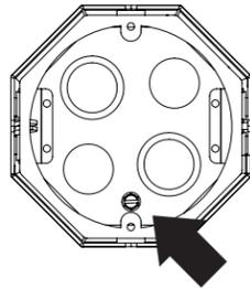
**12** Carefully route wires into junction box and connect module female connector to hardwire adapter male connector.
