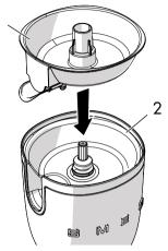
Insert the filter (3) in the juice collector and then place the reamer (4) on top of the filter.
