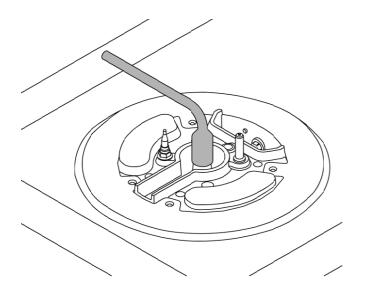
**Step 3: oven burner (main or auxiliary)**To replace the nozzles of the main oven burner, start by removing the door and the bottom panel of the oven.
