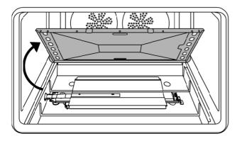
Remove the screw located on the right side of the burner and pull out the burner from its support. ATTENTION: pay extra attention to avoid damage to the igniter and thermocouple.
