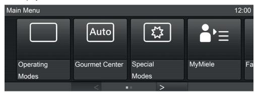
The top line shows what menu level you are currently in. Options within a menu are separated by a vertical line. If there is not enough space to show the whole path, additional options are indicated by ... I. The Time of Day, Alarm 0 and Timer 1 are shown in the top right-hand corner of the display.
