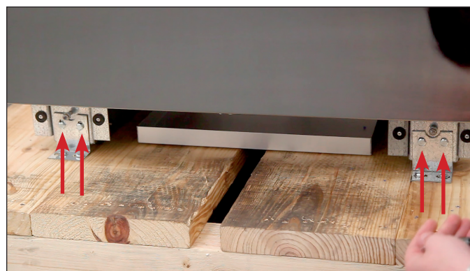
FIG. 7. Shipping bracket bolt locations.
