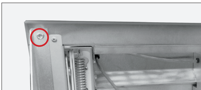
FIG. 8. Bracket screw location. Other bracket not shown.
