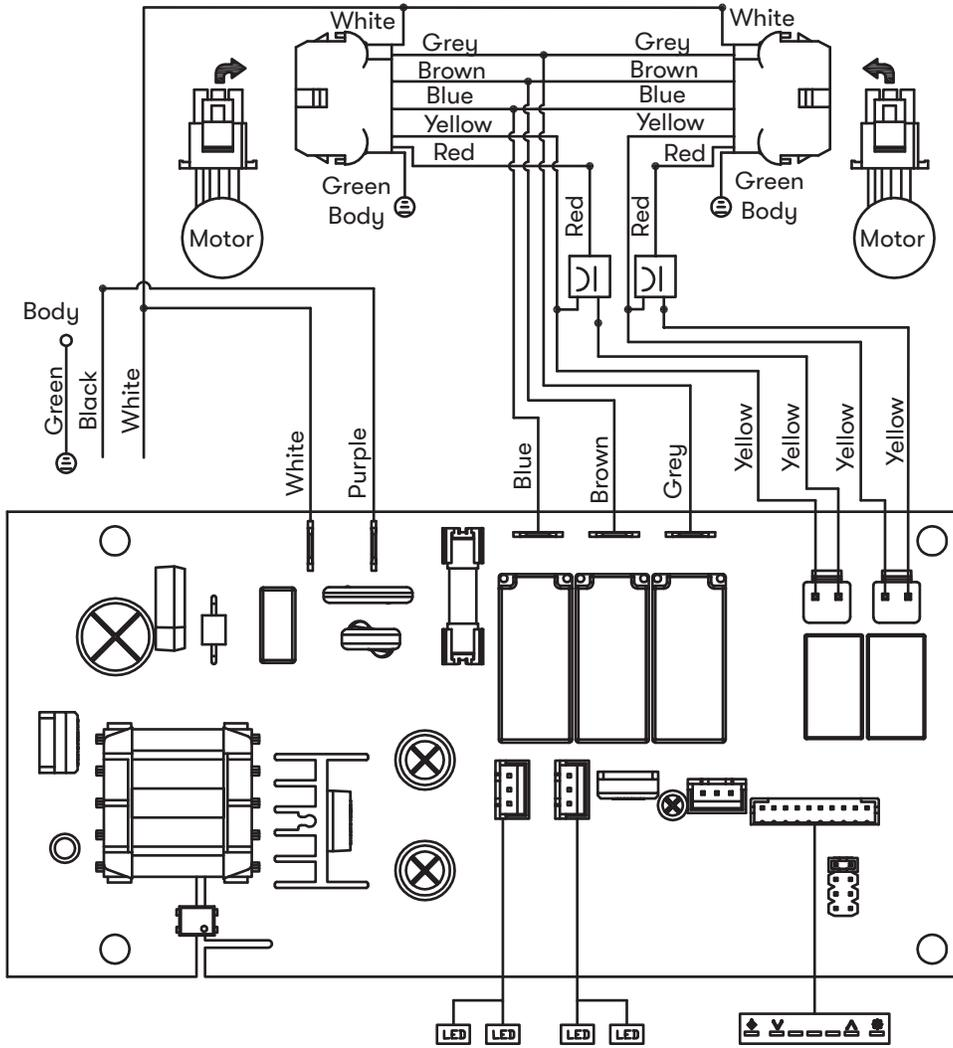
REMARKS: CONDENSER 11+11uF 250VAC \*2 FIT AC120V 60Hz
