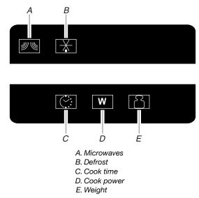
The icons will light up and/or flash in the display while their specific functions are being programmed. The lit icon indicates the function, and the flashing icon is a prompt for input.
