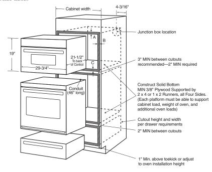
Note: Cabinets installed adjacent 23-1/2" to wall ovens must have an adhesion Cutout depth spec of at least 194° F temperature rating. **⊸** 4-3/16" 25-1/4" Cutout width 21-1/2" Back of Control Junction box location Construct Solid Bottom MIN. 3/8" Plywood Supported by 2 x 4 Conduit 17-1/2" 19" 48-1/2" Cutout height or 1 x 2 Runners. long) all Four Sides. (Platform must be able to support cabinet load, weight of oven. and additional 29-3/4" oven loads) 5" min.from floor 1" min. above toekick
